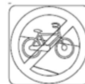
SIGN INDICATING FIFTY METRE (50m) LIMIT OF A BICYCLE CROSSING BLACK PICTOGRAMS, RED CIRCLE & BAR AND GREY ROAD ON WHITE BACKGROUND
