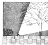
Figure 540-19 Uplighting (directional viewing).
