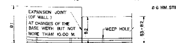
EXPANSION JOINT DETAIL OF WALL
